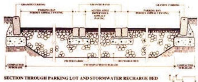
Stormwater Recharge Seepage Bed Section
